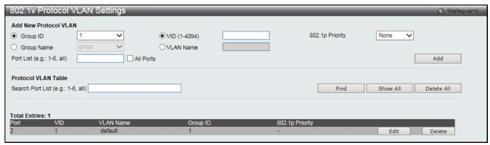
Figure 4-9 802.1v Protocol VLAN Settings window
