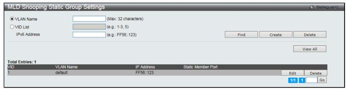
Figure 4-60 MLD Snooping Static Group Settings window
