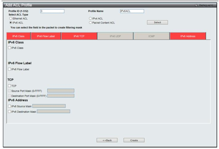
Figure 7-13 Add ACL Profile window (IPv6 ACL)
