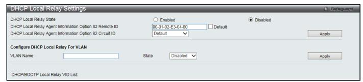
Figure 9-9 DHCP Local Relay Settings window
