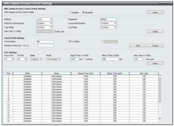
Figure 8-32 MAC-based Access Control Settings window
