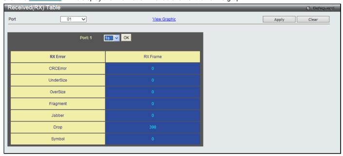
Figure 11-11 RX Error Analysis window (table)
