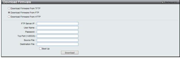
Figure 12-5 Download Firmware - FTP window
