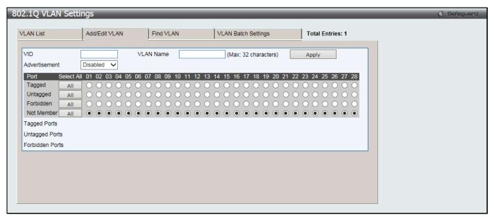
Figure 4-5 802.1Q VLAN Settings - Add/Edit VLAN Tab window
