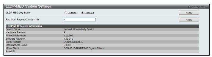
Figure 4-97 LLDP-MED System Settings window
