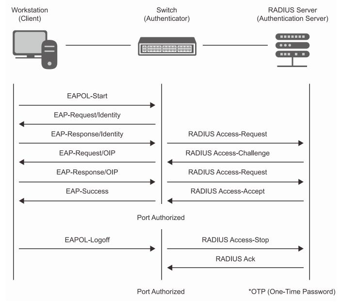
Figure 8-6 The 802.1X Authentication Process
