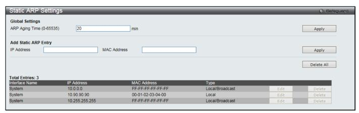
Figure 3-1 Static ARP Settings window
