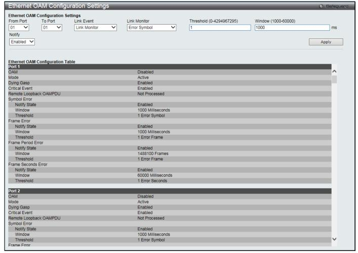
Figure 10-20 Ethernet OAM Configuration Settings window
