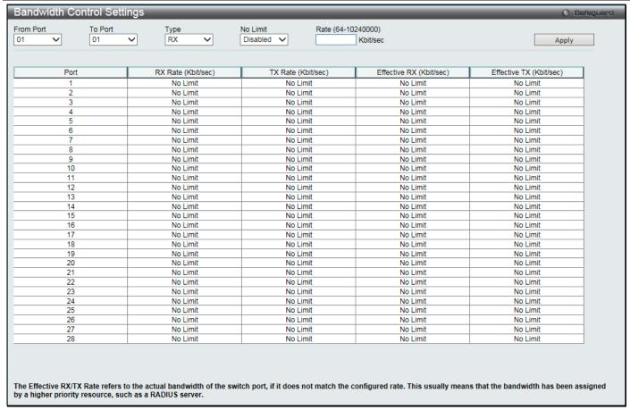
Figure 6-5 Bandwidth Control Settings window
