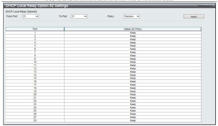
Figure 9-10 DHCP Local Relay Option 82 Settings window
