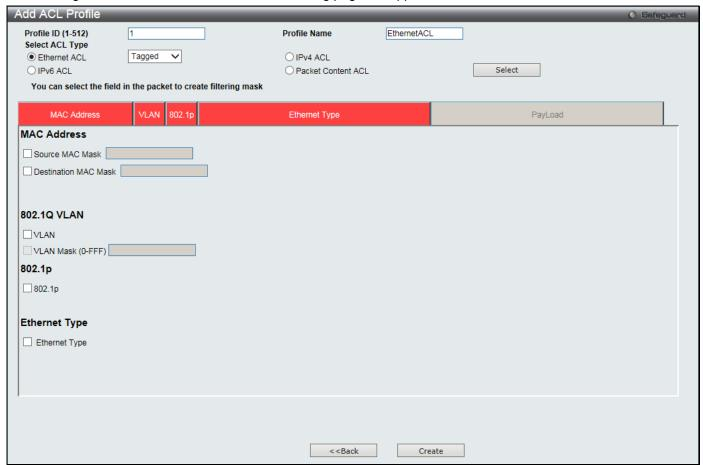
Figure 7-3 Add ACL Profile window (Ethernet ACL)
